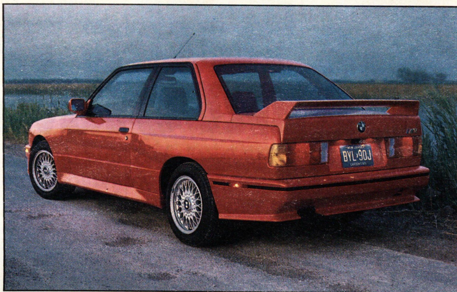
Drag coefficient drops to 0.33 from 0.37 of stock Three Series, a benefit appreciated fully when radar guns aren't present
