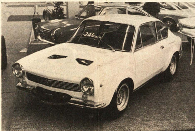
Abarth's latest is the OT 2000, 1.1 is a 2-liter, twin overhead cam, 150 mph tiger. Note spare wheel mounted for use as a bumper. (David Phipps photo)
