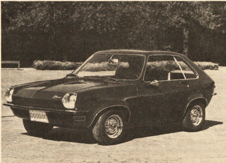
This is a mockup of GM Styling's experimental special purpose commuter car, XP883, as shown May 7 at the GM Progress of Power presentation at the GM Technical Center in Warren, Mich. Designed to carry two adults in front and two children facing the rear, the vehicle can utilize gasoline, electric, or hybrid gasoline-electric power systems.
