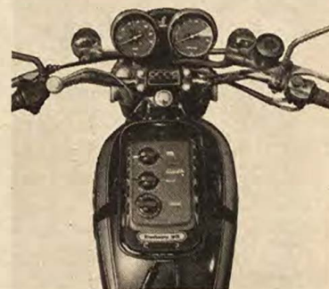
In-helmet headset, optional passenger intercom are features of Beltek Enduro motorcycle model.
