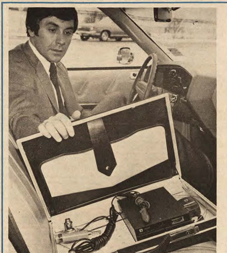
One way to foil thieves is to take equipment with you. Magnetic mount antenna by Antenna specialists Co. teams up here with Johnson set featuring cigarette lighter power source.
