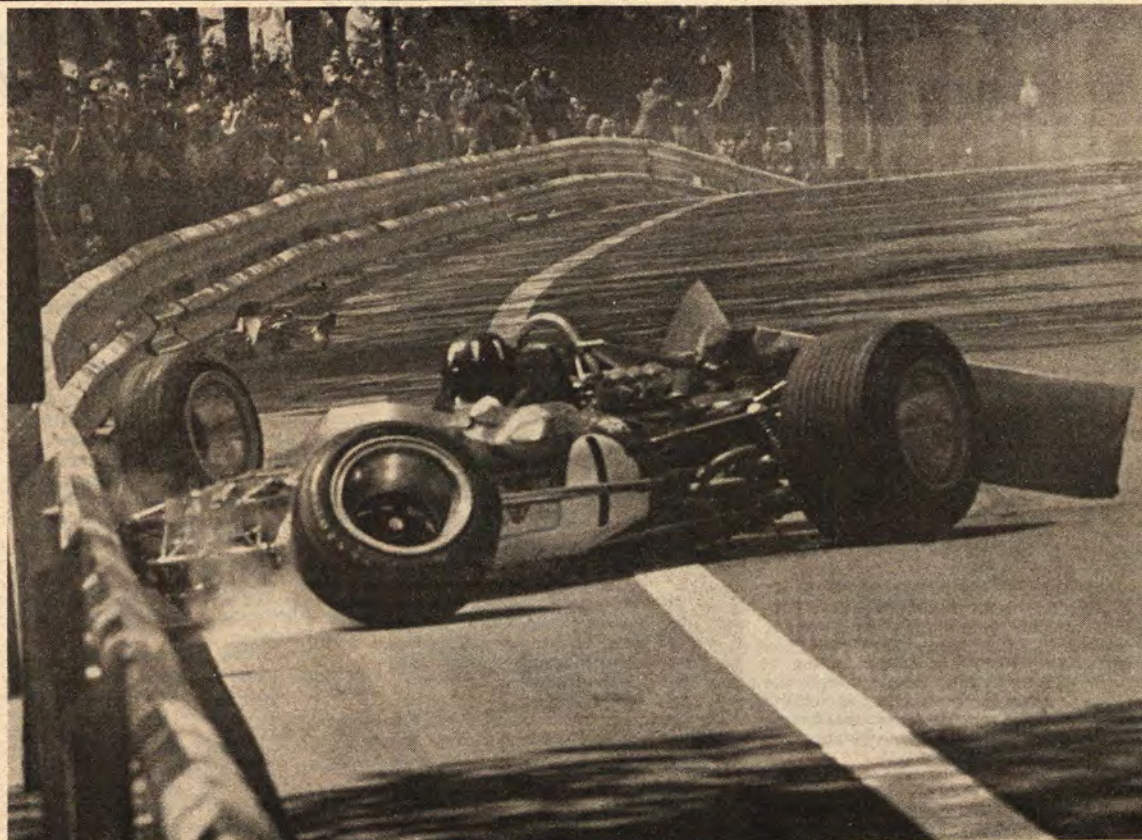
When a wing failed on his Lotus, Graham Hill crashed into the guard railing at Barcelona in 1969; six years later, Rolf Stommelen, driving the Hill GP car, crashed in almost exactly the same spot for the same reason.
