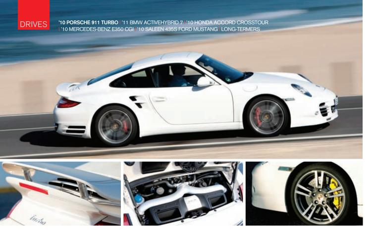
latest evolution of Porsche's flat six-cylinder, with a one-piece crankcase and direct fuel injection, and the optional Porsche-Doppelkupplungsgetriebe (PDK) dualclutch, auto-shift transmission.
